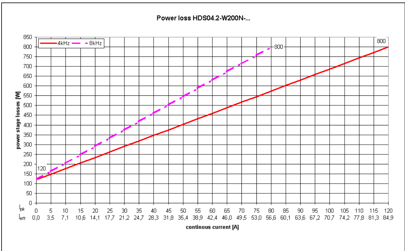
Fig. 7-5: Power loss HDS04.2W0200N-
