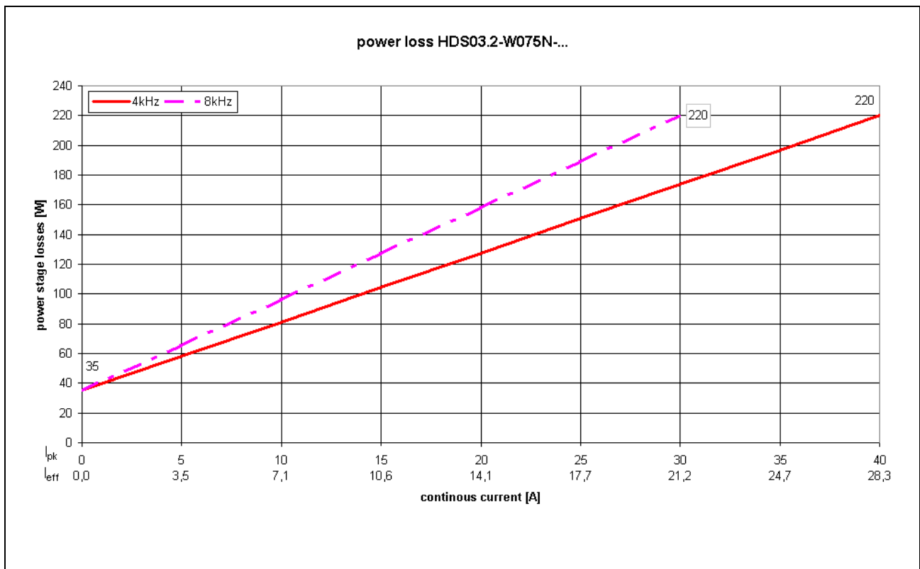
Fig. 7-3: Power loss HDS03.2W075N-
