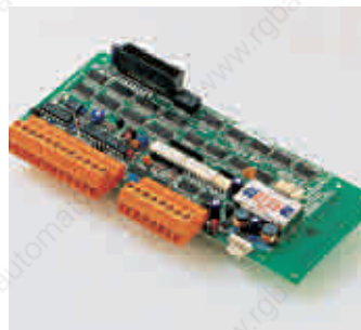
Analogue input board 4 inputs, 10bit resolution
