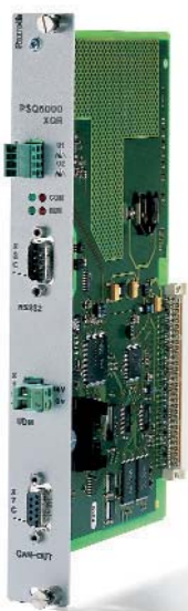
PSQ 6000 control board – for quality in spot welding
