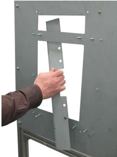
Insert the left reinforcement plate into the mounting cut-out.
