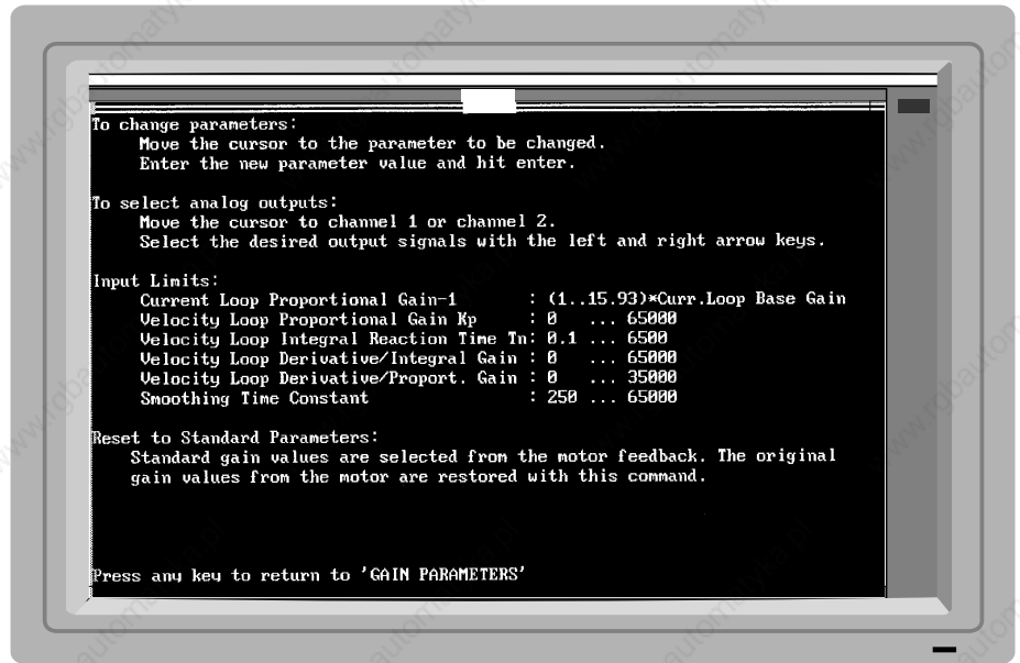
Fig. 54: Help text to "GAIN PARAMETERS" menu
