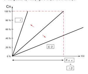
It is possible to optimize the start without modifying its gradual nature by defining an initial torque tq0. The torque reference can be peak limited by tLl.
