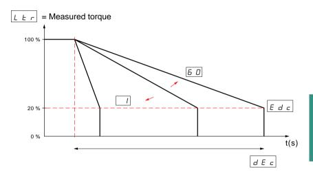
In pump type applications, it is not necessary to control deceleration below a load level set via  $\boxed{\it E~d~c}$ .
