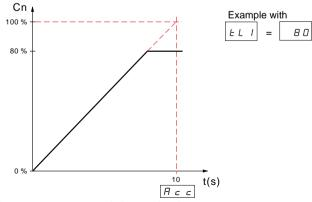
If tLI = tq0: torque constant during acceleration.
