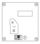
(7) Switches for level 1, 2 and 3 adjustment and configuration, see page 45
