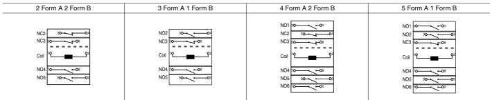
= Reinforced insulation: overvoltage category III, pollution degree 2, 250V AC (Clearance and creepage distance is 5.5 mm .217 inch or more between contact sets shown by "——creepage distance even between contact NO4 and coil.)
