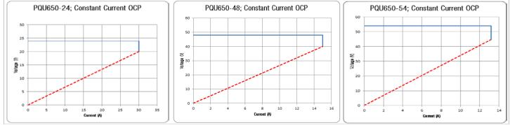
1. Curves generated for the PQU650 variants by subjecting output to an incremental (constant resistance load, equivalent to 1Adc increments (above full load).
