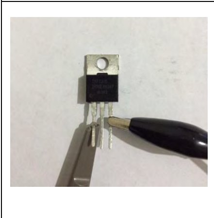
Figure 128: Channel1 Probe Used for Gate - Source Measurement
