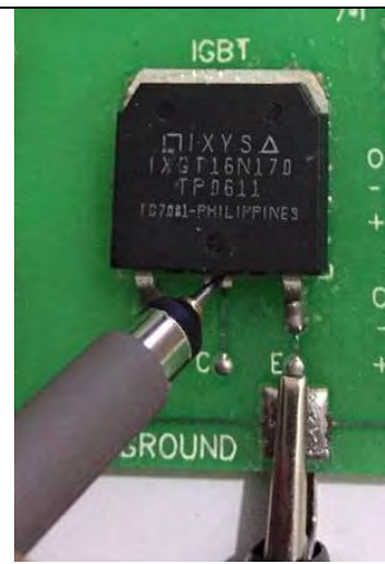
Figure 153: Channel1 Probe Used for Collector - Emitter Measurement
