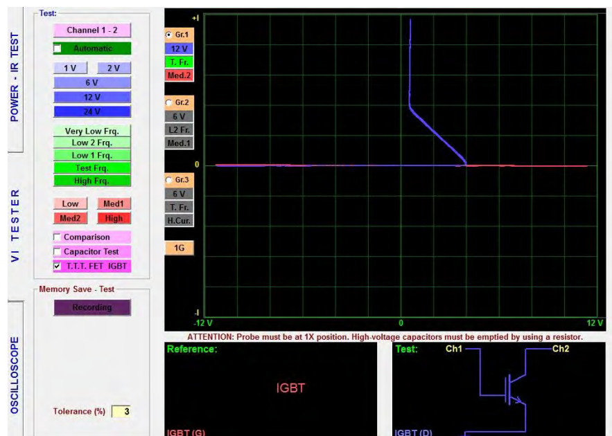
Figure 155: IGBT VI Graph, Equivalent Circuit Diagram
