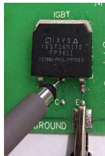
Figure 149: Channel1 Probe Used for Collector - Emitter Measurement
