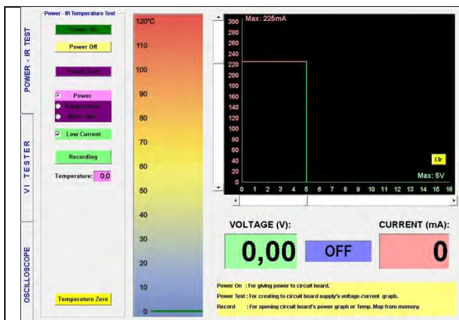
Figure 43: Adjusting the Voltage and Current (Step 1)
