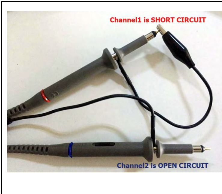
Figure 56: Short Circuit (Channel1) - Open Circuit (Channel2)
