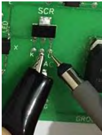
Figure 157: Channel1 Probe Used for Gate - Cathode Measurement
