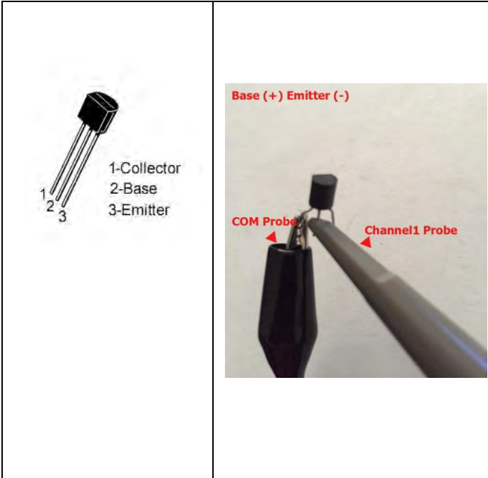
Figure 105: Channel1 Probe used for Base - Emitter Measurement
