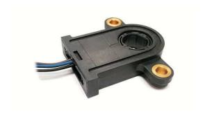
The PST-360 through hole / hollow-shaft position sensors combine three critical design features; 1) through hole where the shaft passes through the sensor, 2) high accuracy absolute position feedback over up to 360 degrees, and 3) a true non-contacting sensing element. Piher's design does not rely on gears or other rotating parts.
