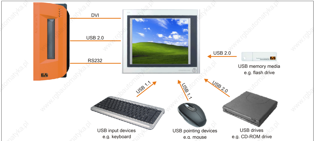
Figure 101: Remote connection of USB peripheral devices on the APC900 via DVI
