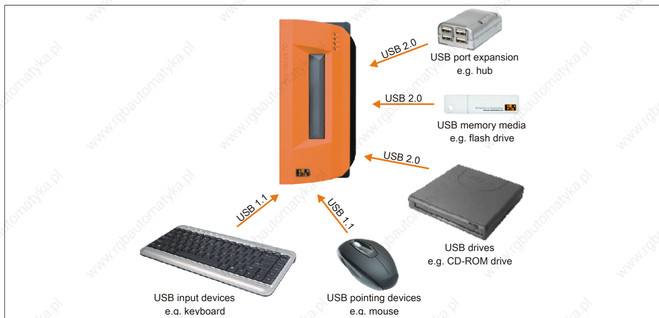
Figure 100: Local connection of USB peripheral devices on the APC810
