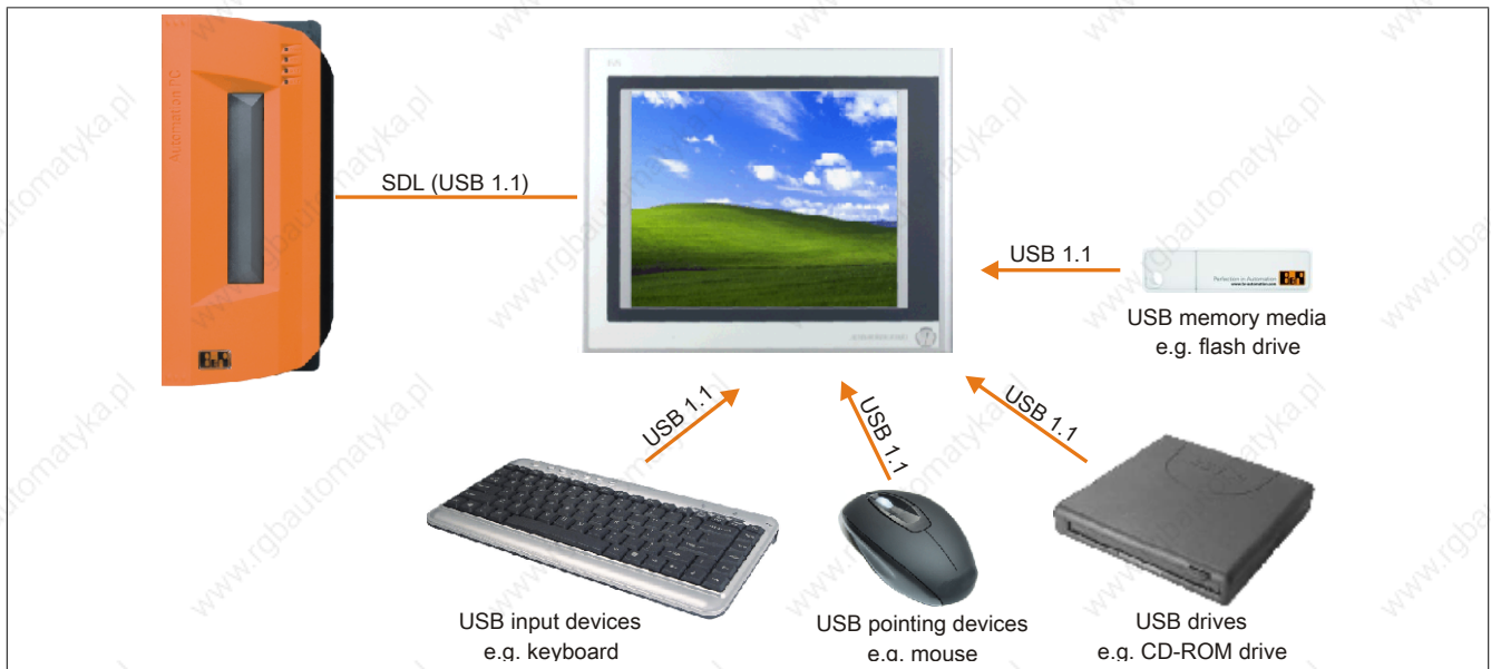
Figure 102: Remote connection of USB peripheral devices on the APC800/900 via SDL
