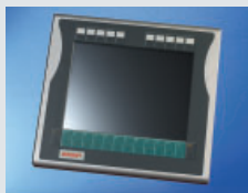
CP77xx | Control Panel, Embedded PC (Pentium®-MMX-compatible CPU, 300 MHz)
