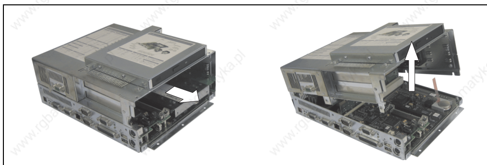
Figure 70: Removing the cover and bus unit
