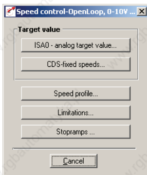
Fig. 8.13 Basic setting "Speed control "OpenLoop", 0-10 V or fixed speeds, control via terminal"
