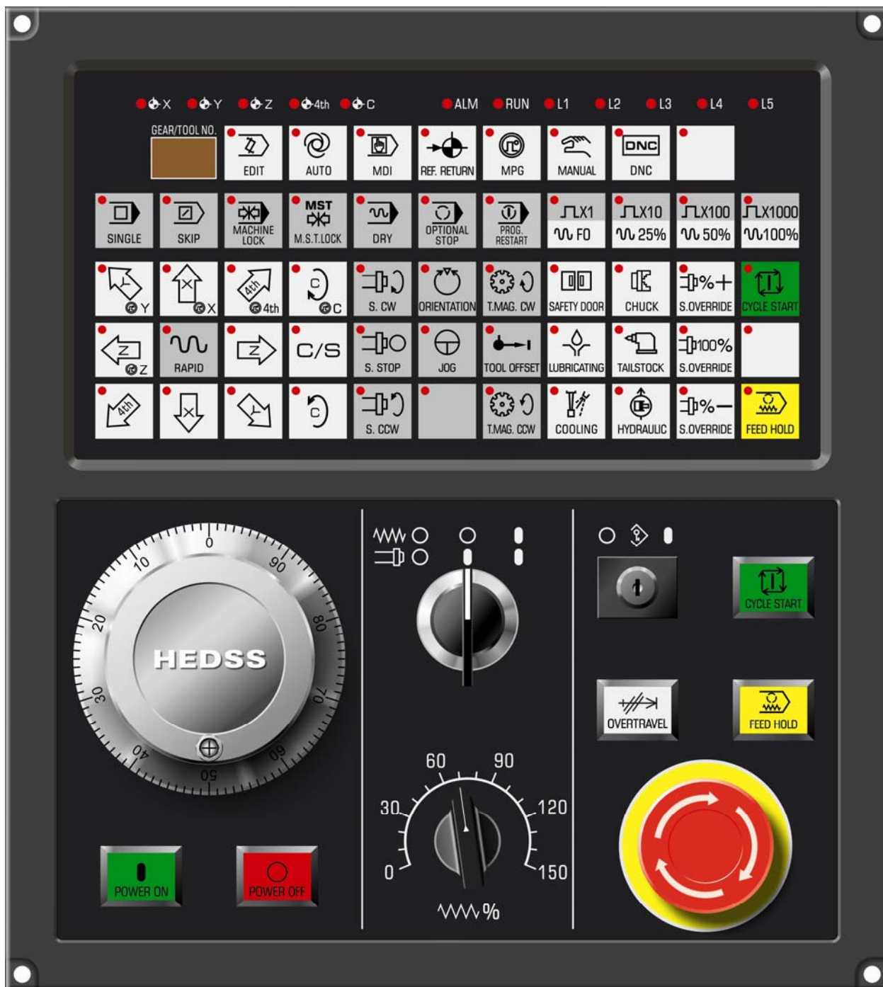
Fig. 6-1-1 Standard layout of operation panel
