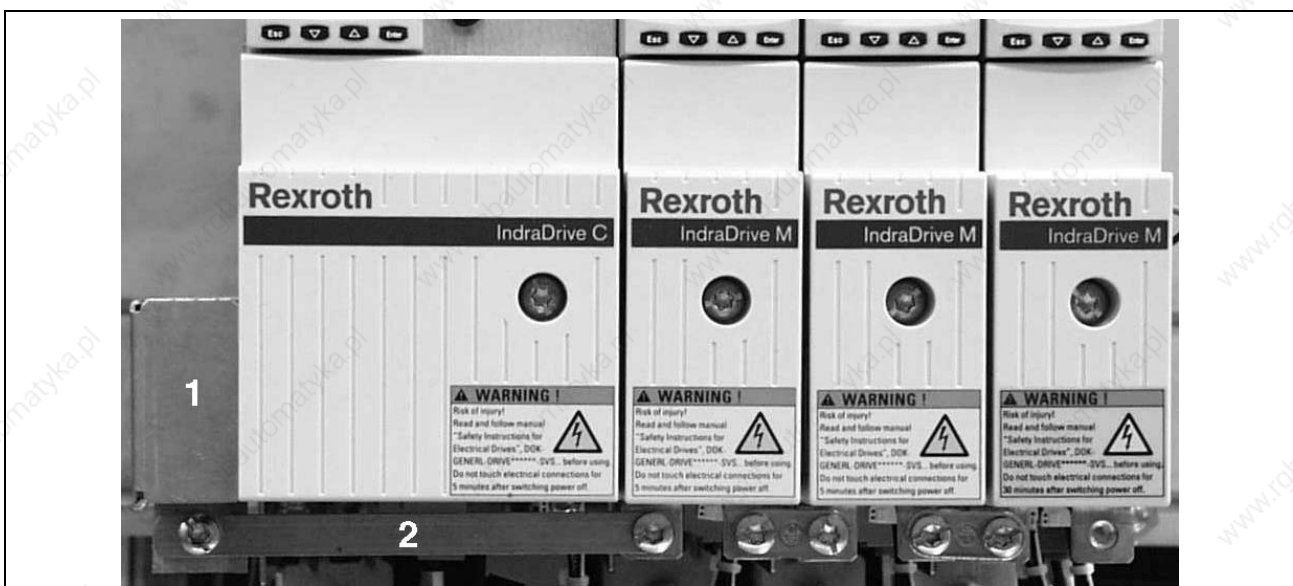
Fig. 14-58: HAS04.1-001 at drive system HCS02 with HMx01 with touch guard mounted
