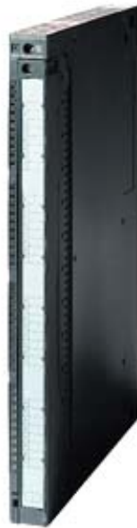
SIMATIC S7-400, SM 422 DIGITAL OUTPUT MODULE, OPTIC. ISOLATED, 32 DO, 24V DC, 0.5A
