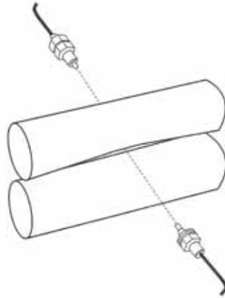
Detecting the roundness of rollers
