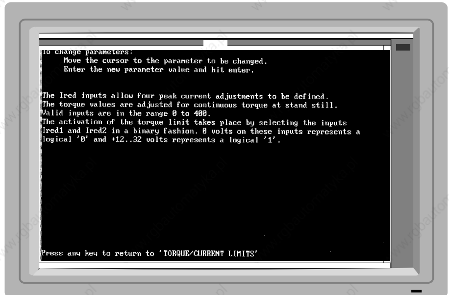
Fig. 52: Help text to "TORQUE/CURRENT LIMITS" menu
