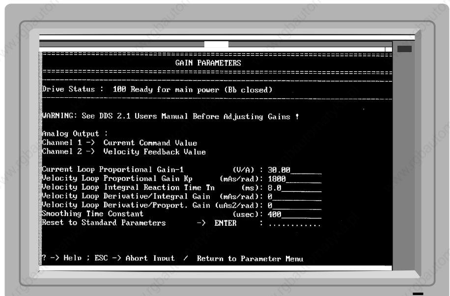
Fig. 53: "GAIN PARAMETERS" menu
