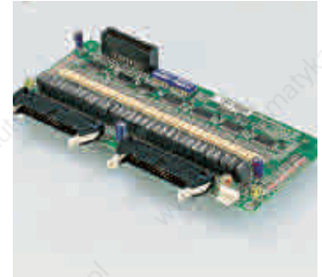
Output board 32 transistor outputs 0.8A
