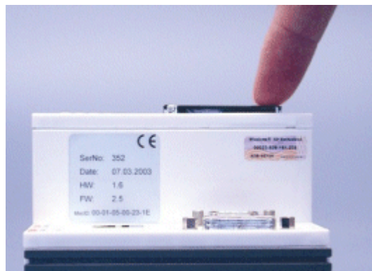
FIG3: Inserting the CF card
