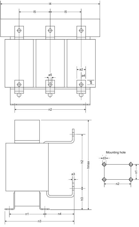
Figure 2-13 Dimension drawing, line reactors
