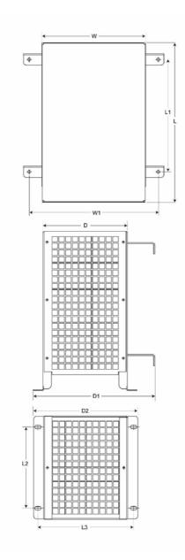
Figure 4-3 Dimension drawing: Braking resistor, frame sizes FSC, FSD, FSE, FSF
