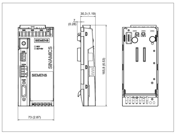
Figure 6-15 Dimension drawing of the CUA32 Control Unit Adapter
