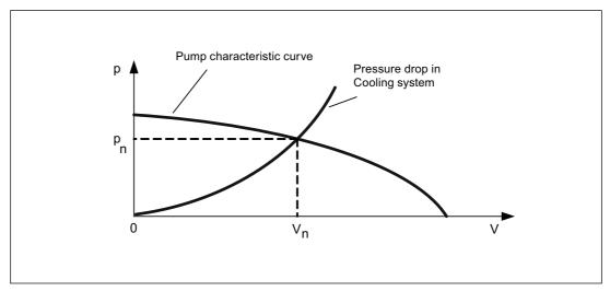
Figure 10-2 Pump characteristic curve
