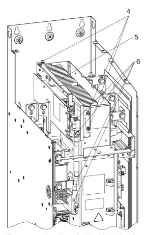
Figure 4-11 Installing a Braking Module in a Power Module, frame size GX – steps 4 - 6
