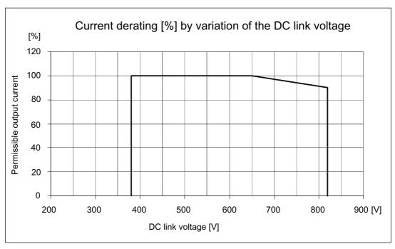
Figure 3-29 Current derating by variation of the DC link voltage
