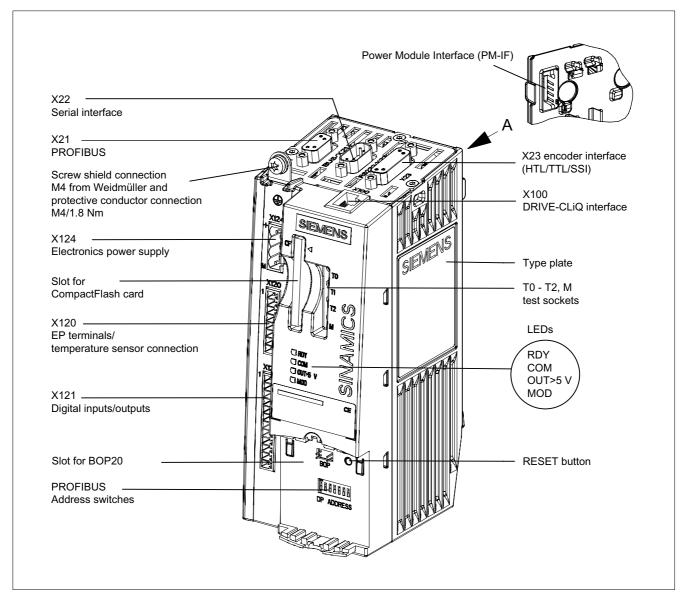
Figure 6-2 Description of the CU310 DP interfaces (ports)
