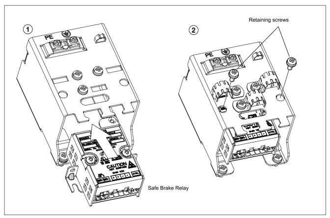
Figure 7-13 Mounting the Safe Brake Relay on the Screening Kit (frame size FSA)
