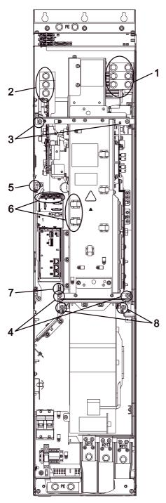
Figure 11-7 Replacing the Powerblock, Power Module, frame size GX
