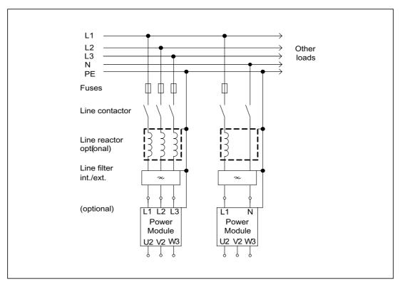
Figure 2-4 Direct operation on the line supply
