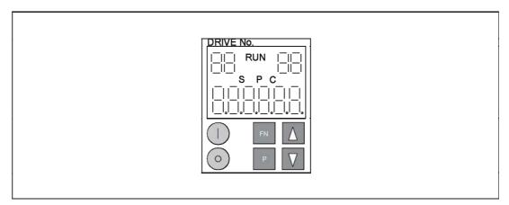
Figure 7-2 Overview of displays and keys
