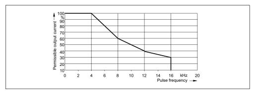
Figure 3-45 Output current as a function of pulse frequency
