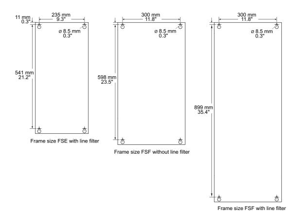
Figure 3-17 Drilling templates for frame sizes FSD to FSF - with and without line filter
