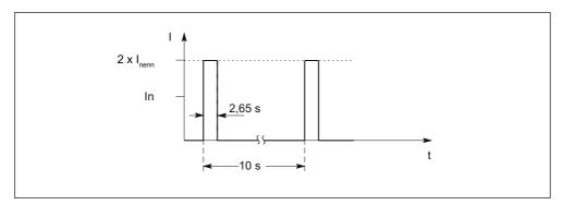
Figure 3-40 Load cycle without pre-load condition (for servo drives)
