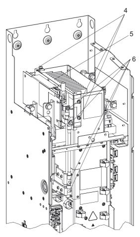
Figure 4-9 Installing a Braking Module in a Power Module, frame size FX – steps 4 - 6
