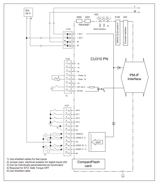
Figure 6-8 Connection example CU310 PN
