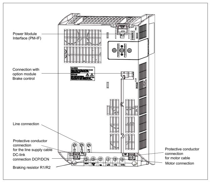
Figure 3-3 PM340, frame size FSC
