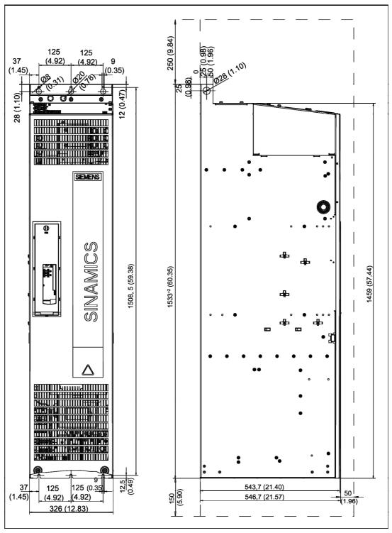
Figure 3-54 Dimension drawing Power Module, frame size GX
