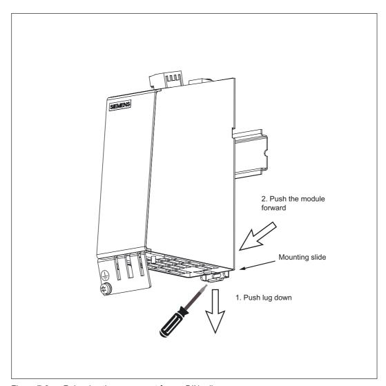
Figure 7-6 Releasing the component from a DIN rail
