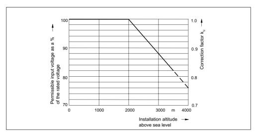
Figure 3-61 Voltage correction factor as a function of installation altitude
