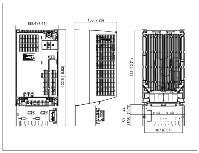
Figure 8-11 Dimension drawing: Power Module PM340 with Screening Kit and Brake Relay, frame size FSC
