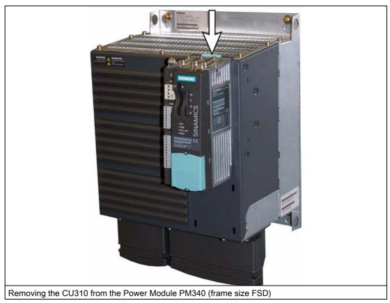
In order to remove the Control Unit from the Power Module, the blue release lever, as shown in the diagram, must be pressed downwards and the Control Unit swung-out to the front.
