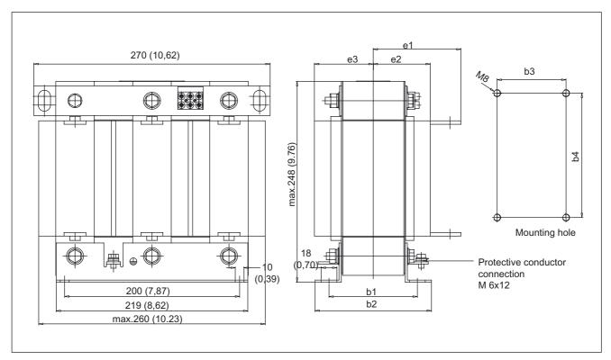
Figure 5-4 Dimension drawing: Motor reactor, frame size FSE
