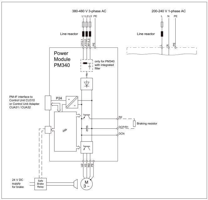
Figure 3-7 PM340 connection example
