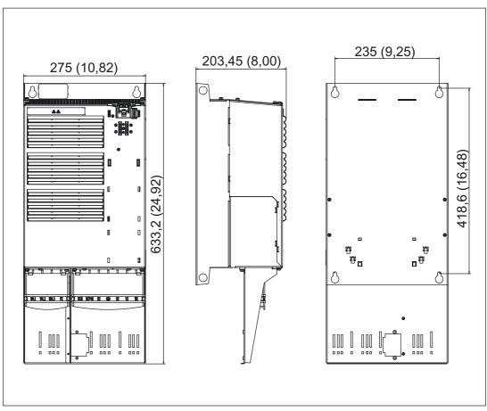
Figure 8-15 Dimension drawing: Power Module PM340 with Screening Kit, frame size FSD
