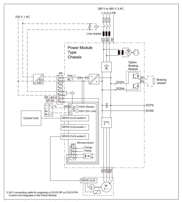
Figure 3-52 Connection example: Power Module Chassis
