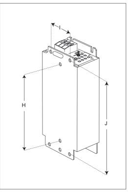
Figure 2-14 Mounting: Line reactor, frame size FSA
