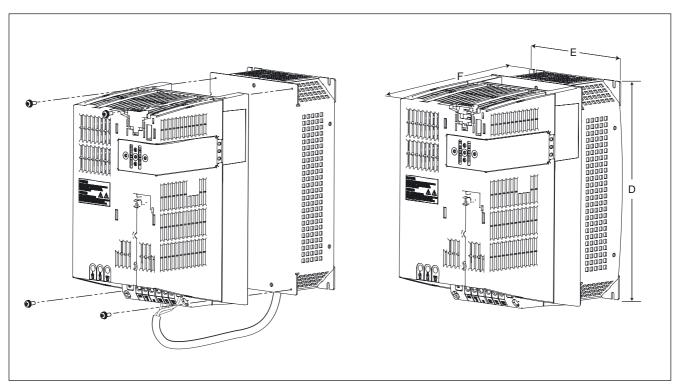
Figure 5-9 Mounting Power Modules and motor reactors, frame sizes FSB and FSC
