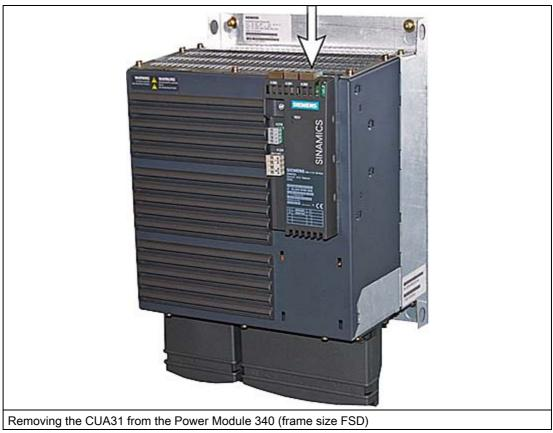
In order to remove the Control Unit Adapter CUA31 from the Power Module, the blue release lever, as shown in the diagram, must be pressed downwards and the Control Unit Adapter CUA31 is swung-out to the front.
