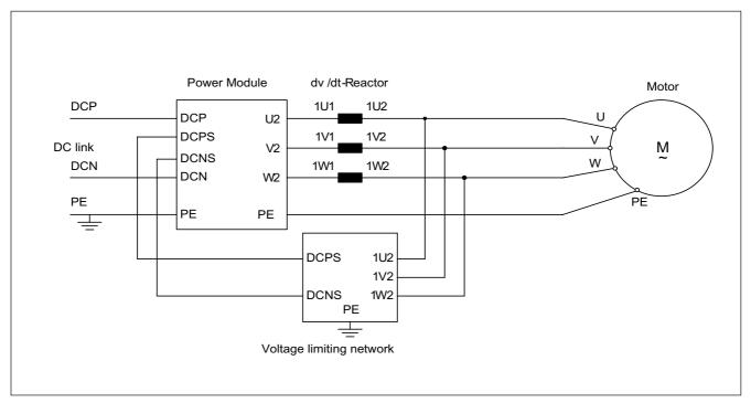
Figure 5-15 Connecting the dv/dt filter with Voltage Peak Limiter
