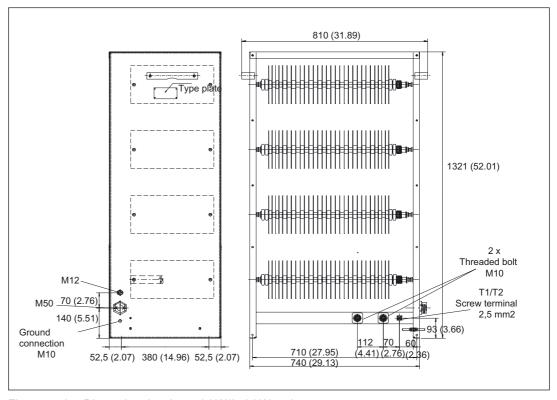
Figure 4-13 Dimension drawing, 50 kW/250 kW resistor
