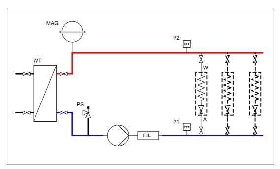
Figure 10-1 Example: Closed cooling circuit
