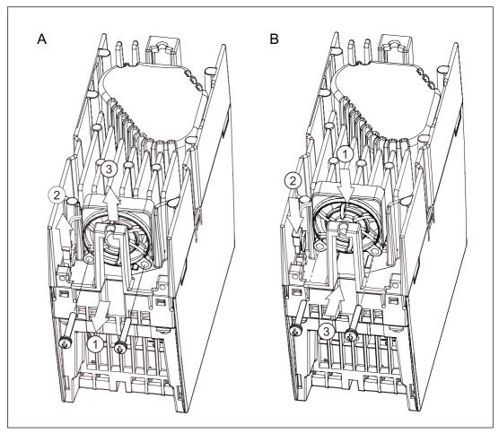
Figure 11-1 Replacing the fan for a Power Module PM340, frame size FSA (tightening torque 0.4 Nm)
