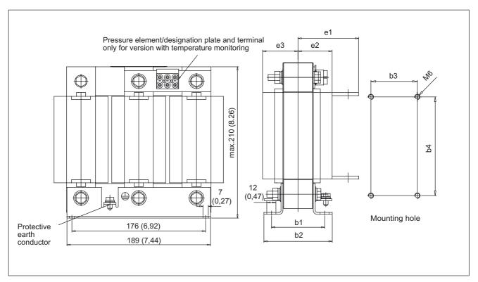
Figure 5-3 Dimension drawing: Motor reactor, frame size FSD
