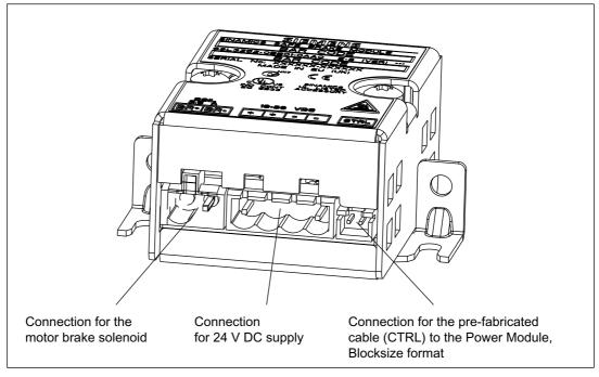
Figure 7-10 Interface description: Safe Brake Relay
