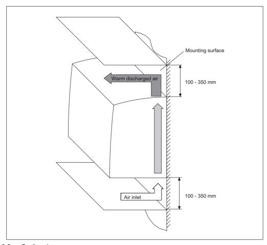
Figure 9-3 Cooling clearances
