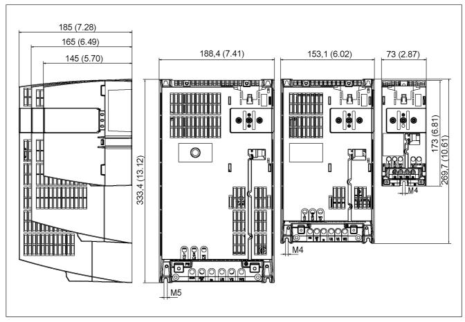
Figure 3-9 Dimension drawings, Power Module PM340
