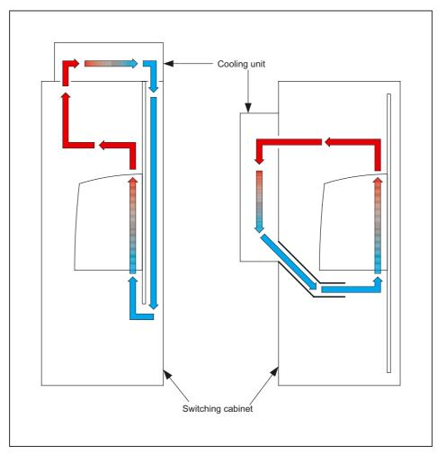
Figure 9-4 Examples of cabinet ventilation
