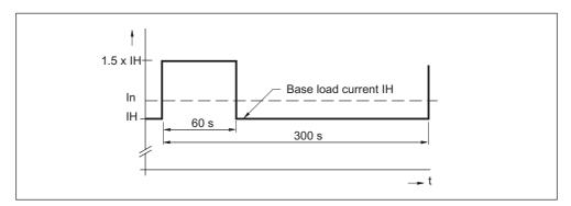
Figure 3-23 Load cycle with 60 s overload with a load cycle period of 300 s
