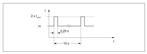
Figure 3-19 Load cycle with pre-load condition (for servo drives)
