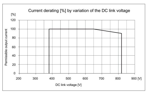
Figure 3-49 Current derating by variation of the DC link voltage
