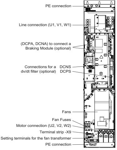
Figure 3-51 Power Module, frame size GX
