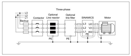
Figure 2-1 Example of a blocksize line connection
