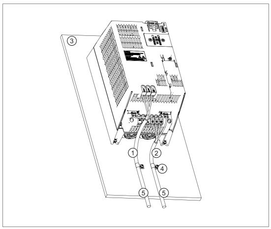
Figure 9-2 Shielding of a Power Module PM340
