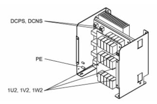
Figure 5-13 Interface overview, voltage limiting network, type 1
