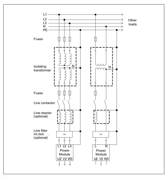
Figure 2-6 Isolating transformer
