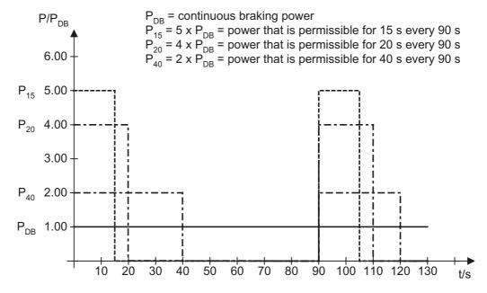
Figure 4-14 Duty cycle for braking resistors
