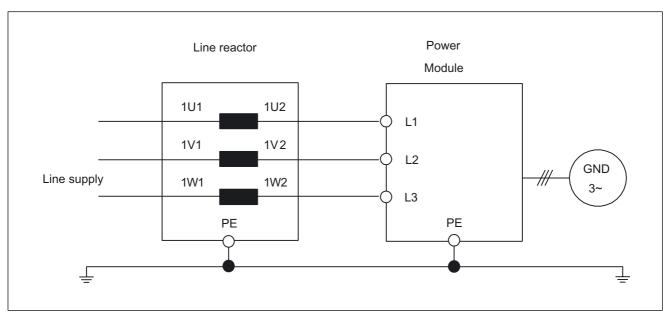
Figure 2-18 Power Module with line filter
