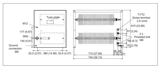
Figure 4-12 Dimension drawing, 25 kW/125 kW resistor
