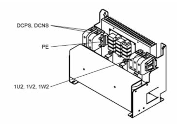
Figure 5-14 Interface overview, voltage limiting network, type 2
