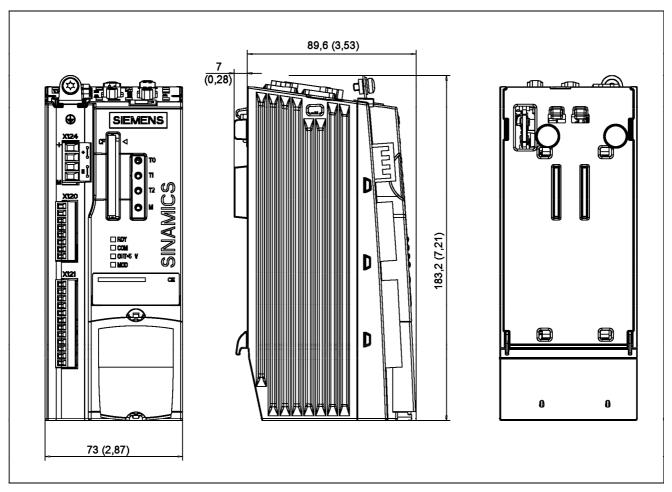
Figure 6-9 Dimension drawing, CU310 PN
