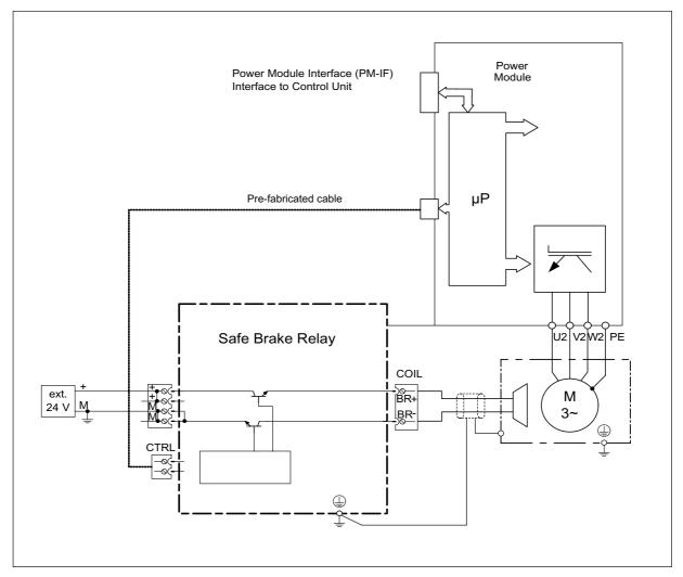
Figure 7-11 Connection example: Safe Brake Relay
