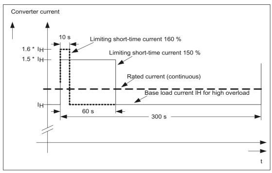
Figure 3-58 High overload
