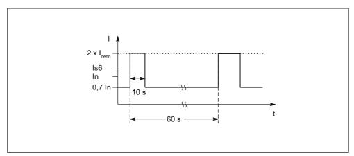
Figure 3-42 Load cycle with pre-load condition (for servo drives)
