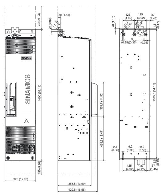
Figure 3-53 Dimension drawing Power Module, frame size FX
