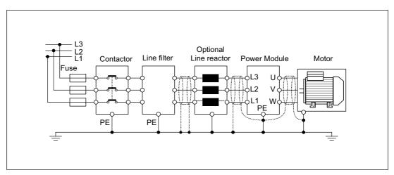
Figure 2-2 Example of a chassis line connection
