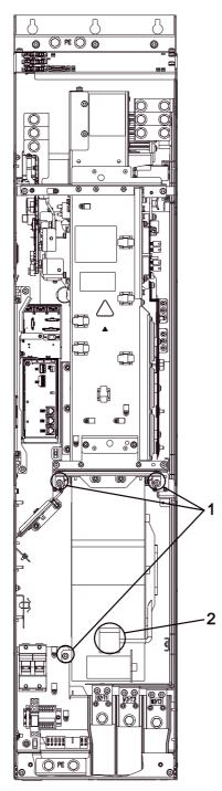
Figure 11-9 Replacing the fan, Power Module, frame size GX
