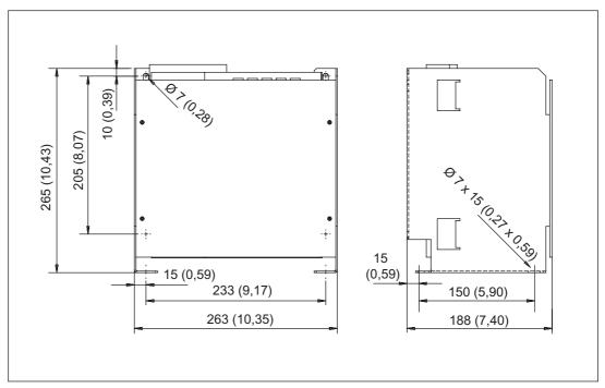
Figure 5-17 Dimension drawing of Voltage Peak Limiter, type 1
