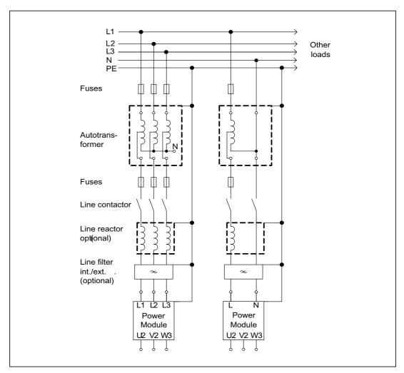
Figure 2-5 Autotransformer
