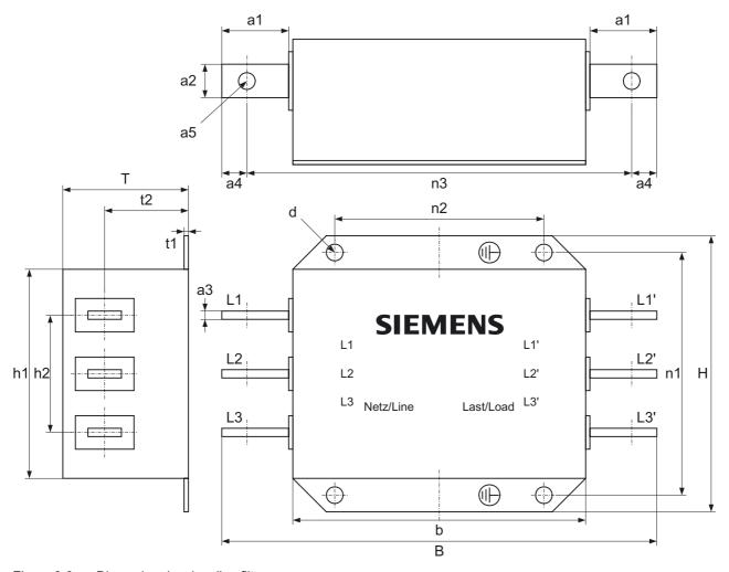
Figure 2-8 Dimension drawing, line filter
