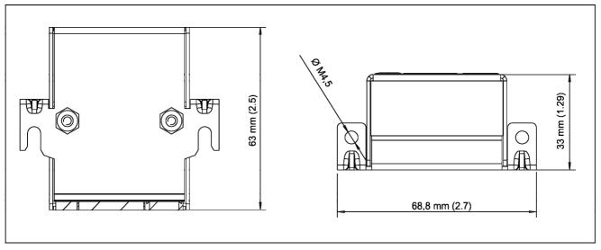
Figure 7-12 Dimension drawing: Safe Brake Relay
