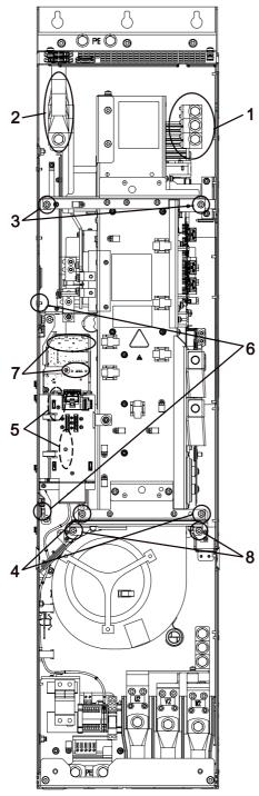
Figure 11-6 Replacing the Powerblock, Power Module, frame size FX
