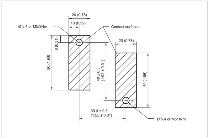
Figure 8-7 Hole drilling template for installation
