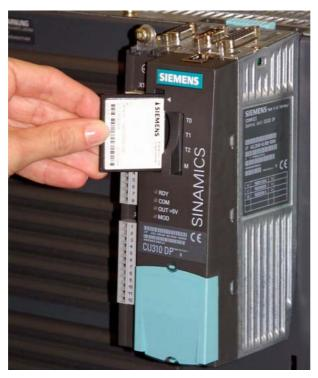
Figure 6-4 Slot for CompactFlash card
