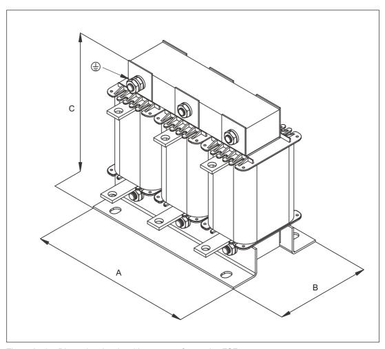
Figure 2-12 Dimension drawing: Line reactor, frame size FSF
