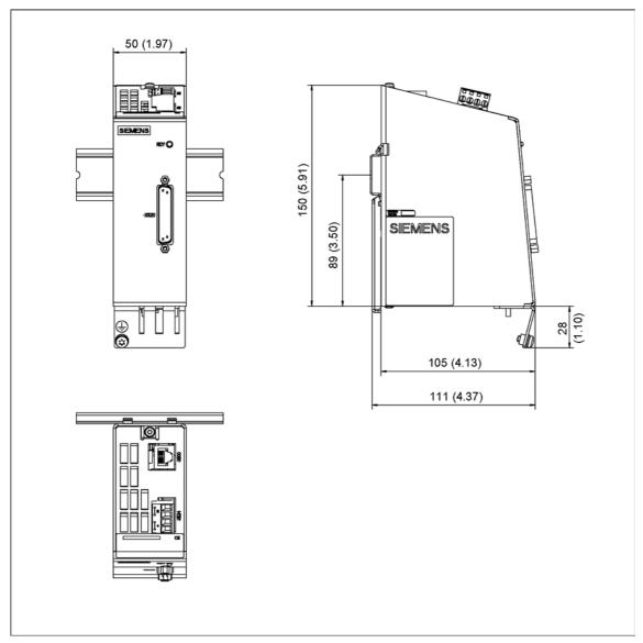
Figure 7-8 Dimension drawing of the SMC20
