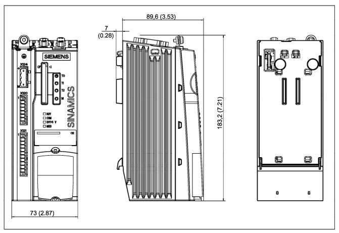
Figure 6-5 Dimension drawing CU310 DP
