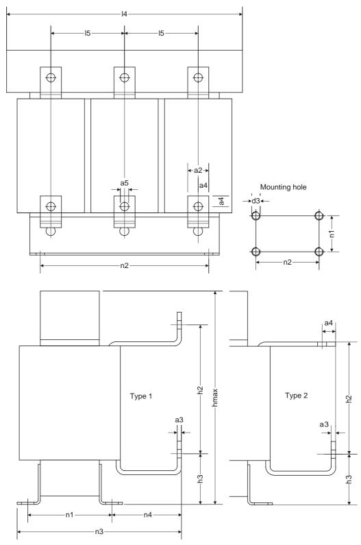
Figure 5-11 Dimension drawing, motor reactor
