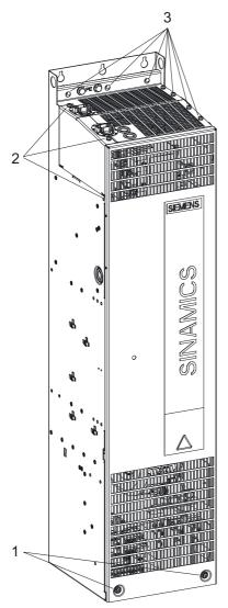
Figure 4-8 Installing a Braking Module in a Power Module, frame size FX – steps 1 - 3
