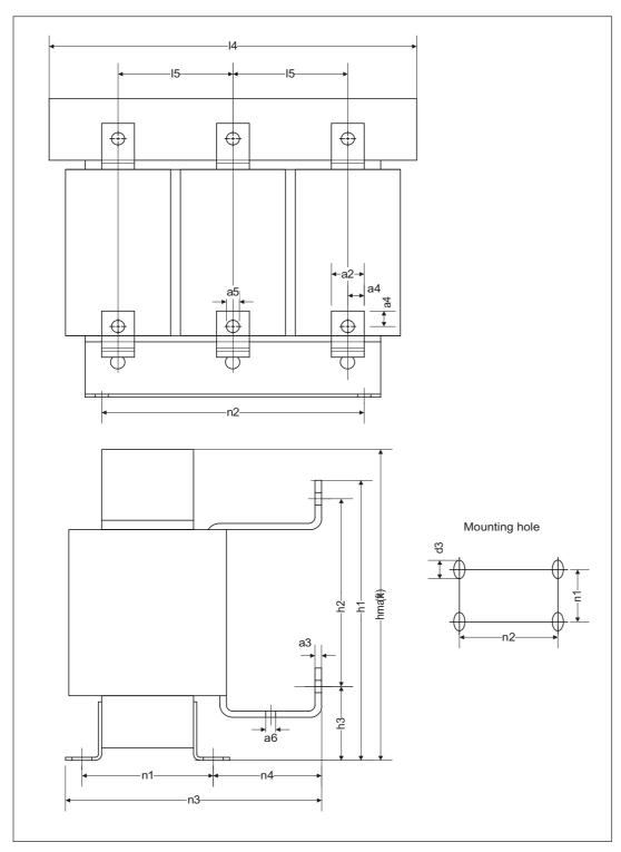
Figure 5-16 Dimension drawing, dv/dt reactor
