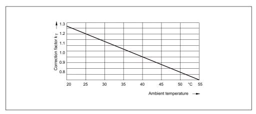
Figure 3-59 Current correction factor as a function of ambient temperature
