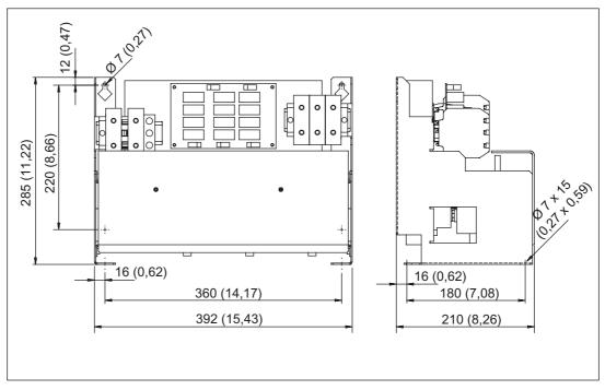
Figure 5-18 Dimension drawing of Voltage Peak Limiter, type 2
