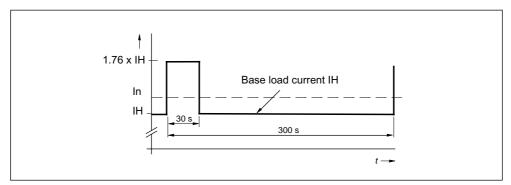
Figure 3-44 Load cycle with 30 s overload with a load cycle period of 300 s
