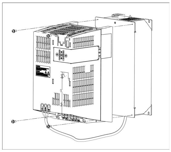
Figure 2-16 Mounting: PM340 and line reactor, frame size FSB
