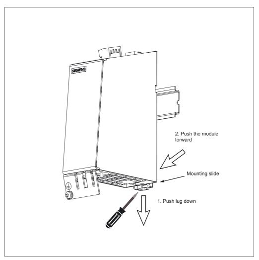
Figure 7-9 Releasing the component from a DIN rail
