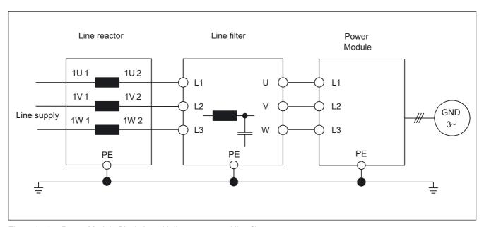
Figure 2-19 Power Module Blocksize with line reactor and line filter
