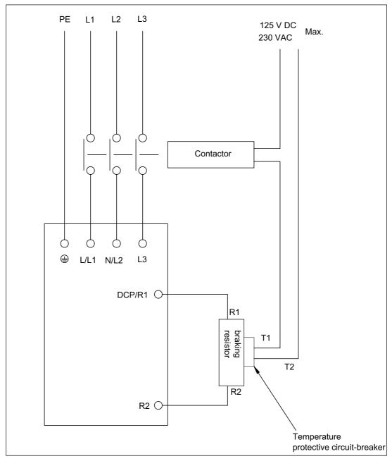
Figure 4-1 Connection example: Braking resistor
