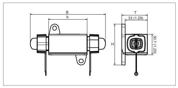
Figure 8-6 Dimension drawing, DRIVE-CLiQ coupling
