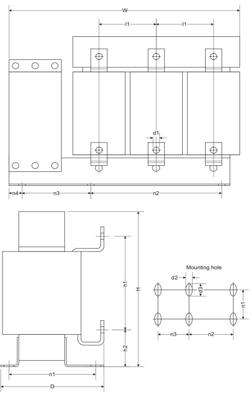
Figure 5-12 Dimension drawing, sinusoidal filter
