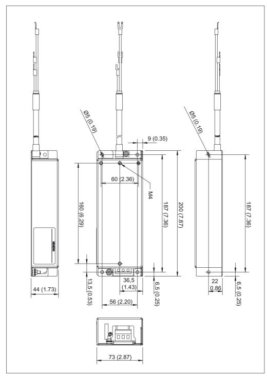
Figure 2-7 Dimension drawing: Line filter, frame size FSA
