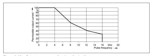
Figure 3-25 Output current as a function of pulse frequency
