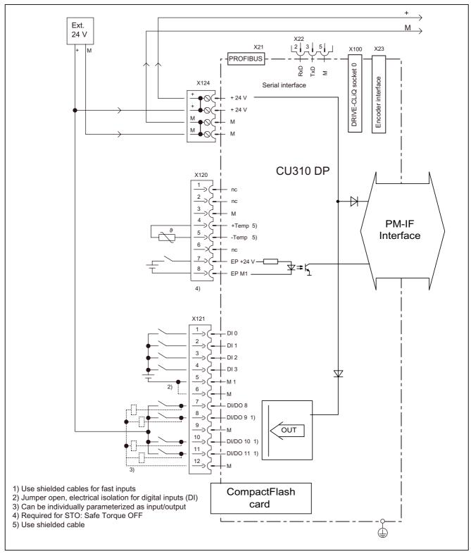
Figure 6-3 Connection example CU310 DP
