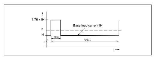
Figure 3-24 Load cycle with 30 s overload with a load cycle period of 300 s
