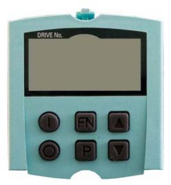
Figure 7-1 Basic Operator Panel BOP20
