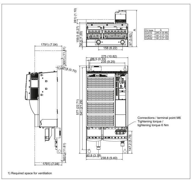
Figure 3-34 Dimension drawing: Power Module PM340, frame size FSE Liquid Cooled
