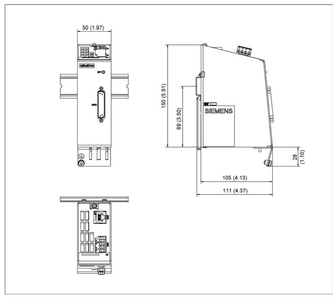
Figure 7-5 Dimension drawing of the SMC10
