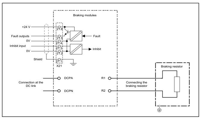
Figure 4-7 Example connection of Braking Module
