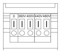
Figure 3-56 Setting terminals for the fan transformers
