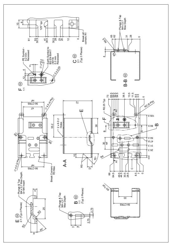
Figure 8-12 Dimension drawing: Screening Kit, frame size FSA
