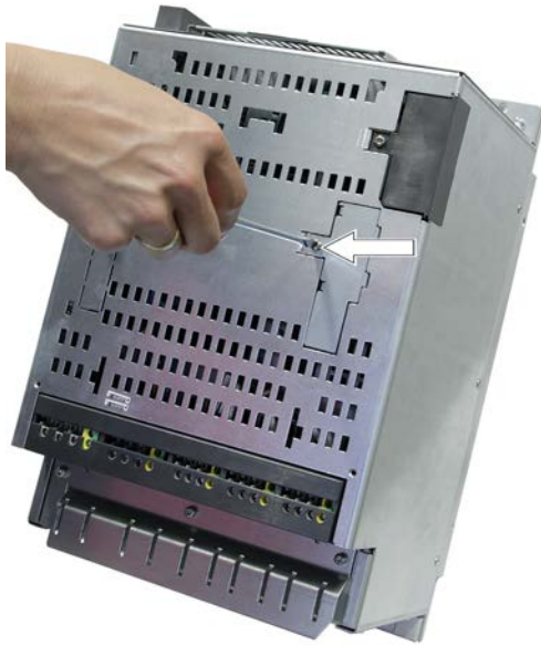
2. Remove the Torx-slotted screw from the fan cover.
