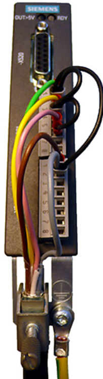
Figure 8-16 Photo of connection example 2: SMC30, 30 mm wide
