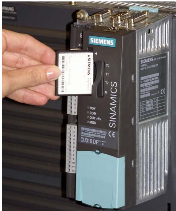
Figure 6-5 Slot for CompactFlash card
