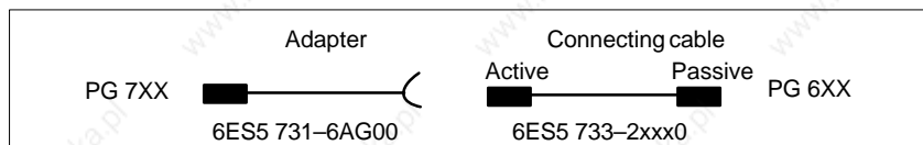
Figure 4-9 Direction of Connection: Adapter – Connecting Cable
