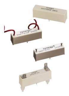
Very high isolation voltages, up to 15kV. are achieved through the use of high vacuum reed switches with either Rhodium or Tungsten contacts and make these relays suitable for high reliability applications, such as cardiac defibrillators, test equipment and high voltage power supplies.
