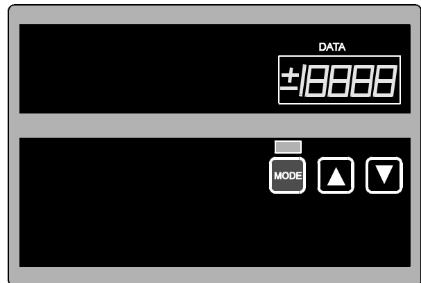
Figure 5-2 Control Keypad used in models SA038, SA059, SA091, SA110, SA150
