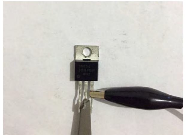
Figure 133: Channel1 Probe Used for Drain - Source Measurement
