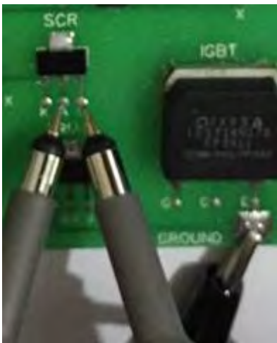
Figure 163: Channel1 (+), Channel2 (+), COM (-) Thyristor Test
