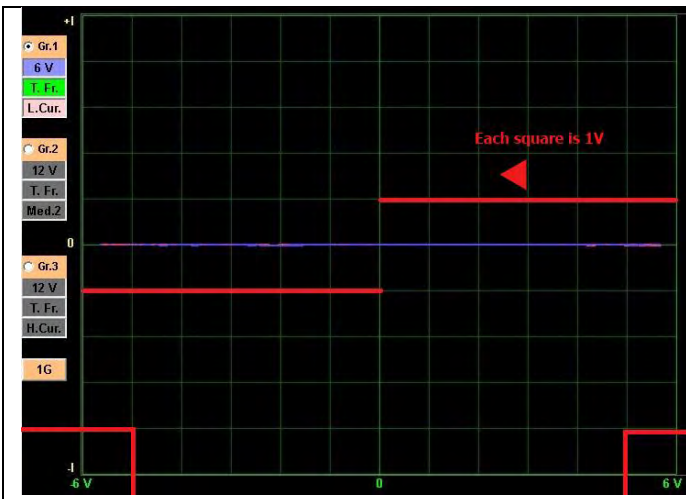
Figure 59: If the Test Voltage 6V, Each Square Represents 1V.
