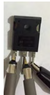
Figure 144: Sample of a Defective N Channel FET
