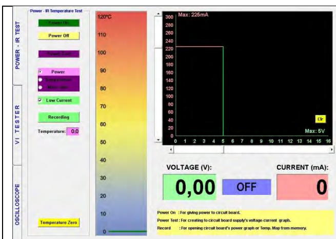
Figure 32: Adjusting the Voltage and Current (Step 1)
