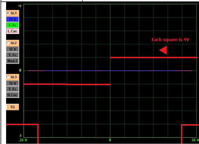
Figure 59: If the Test Voltage 6V, Each Square Represents 1V.
