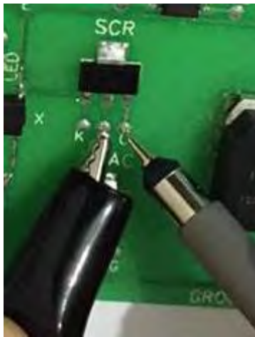
Figure 157: Channel1 Probe Used for Gate - Cathode Measurement
