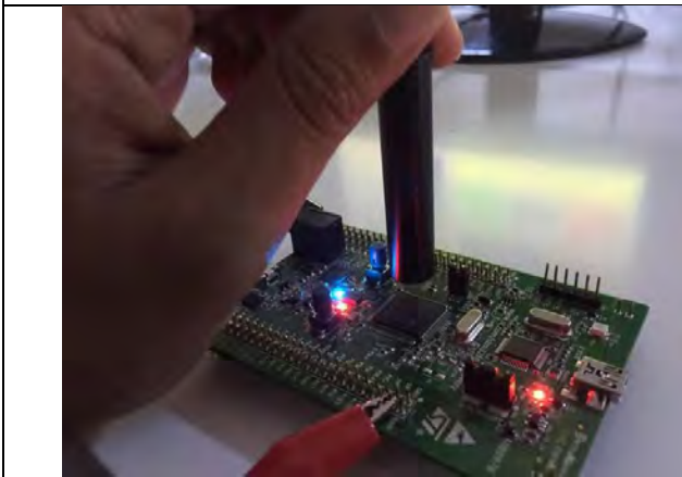
Figure 49: IR Sensor Component Temperature Measurement (Step 7)
