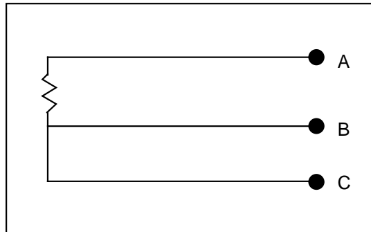
Figure 8-1 RTD Calibration Connection
