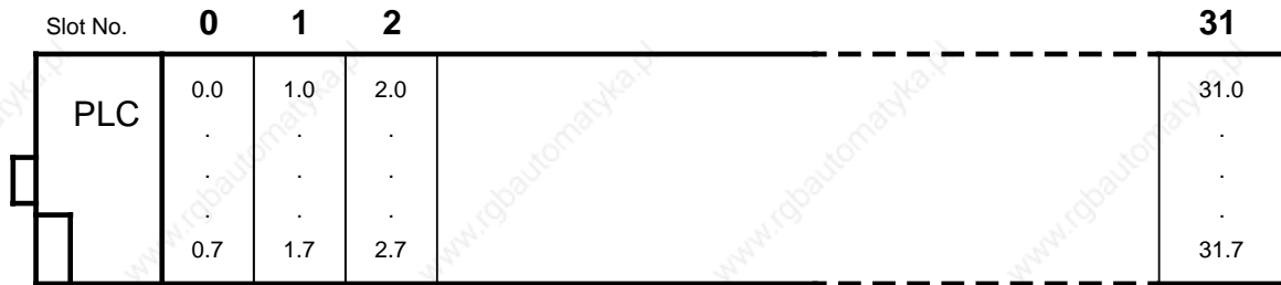
Figure 6-5. Address Assignments for Digital Modules with Four or Eight Channels
