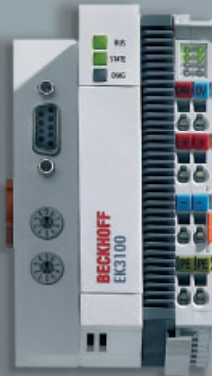
Bus Coupler, e.g. PROFIBUS, PROFINET
