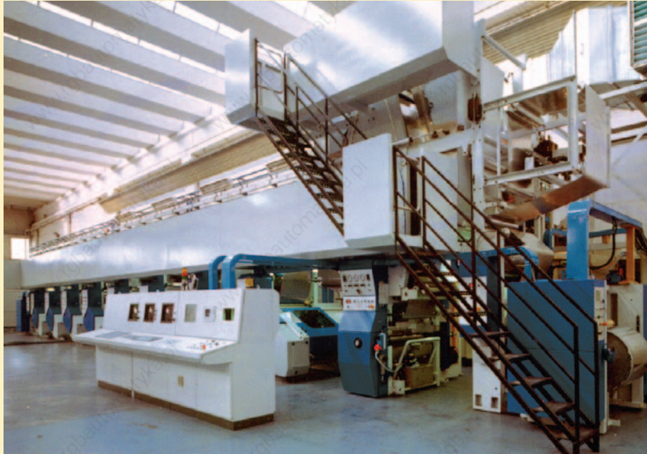
Precision drive-to-drive synchronisation with CTSync on the Unidrive has revolutionised the printing industry with new, "jitter free" 8- and 10-colour flexographic presses. Retrofits with this gearless technology are giving older presses new life and greater flexibility.
