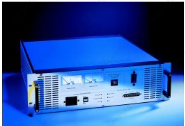
DC - AC Sine-wave inverter 2500VA
