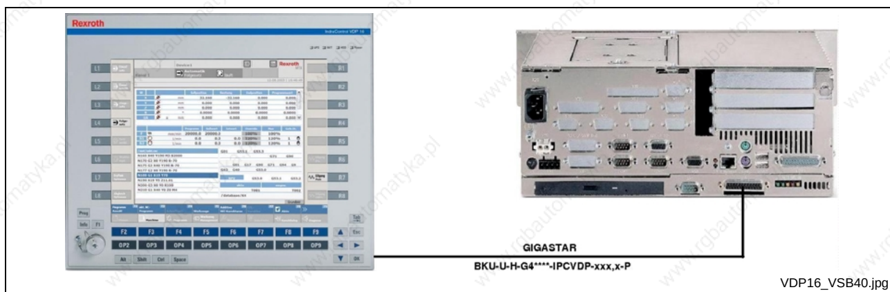
Fig. 6-1: Standard industrial PC VSB 40.1 with operator panel VDP 16.1
