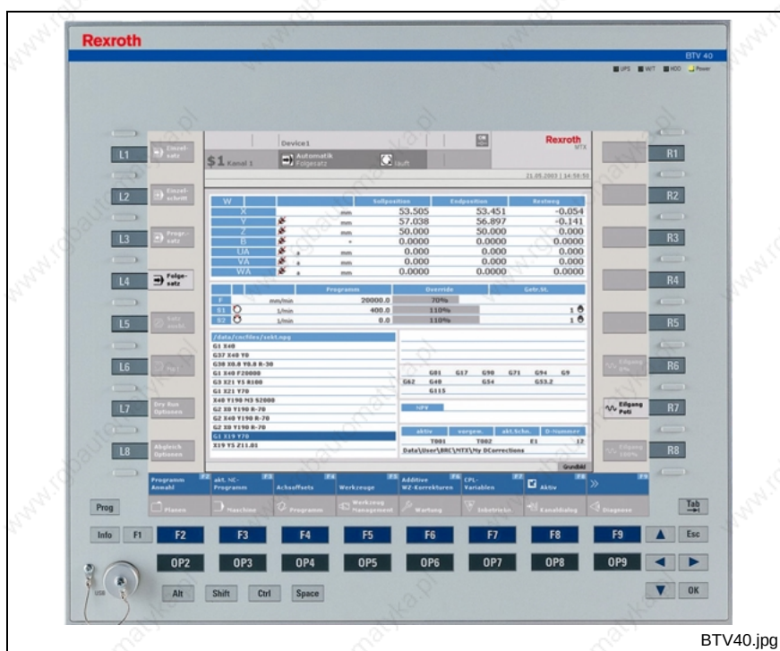
Fig. 7-2: High-end industrial PC BTV 40.2 / VPP 40.1 with 15" color display
