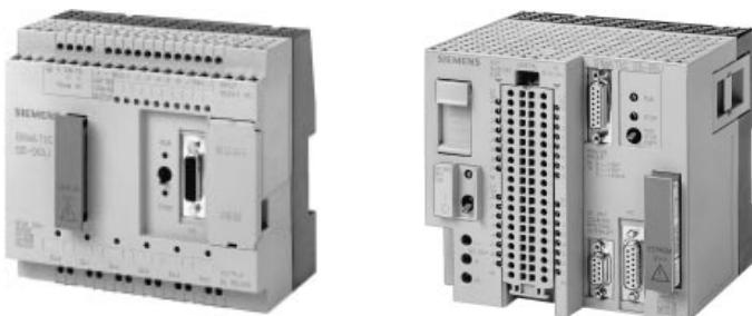
The S5-90U and S5-95U consist of a tough plastic case, into which the processor, power supply, inputs and outputs are integrated. This enclosure can be snapped onto a DIN rail. Both devices can be expanded with all I/O modules of the S5-100U. The S5-90U is expandable over the IM 90 interface, the S5-95U is directly expandable (see also page 2/3).
