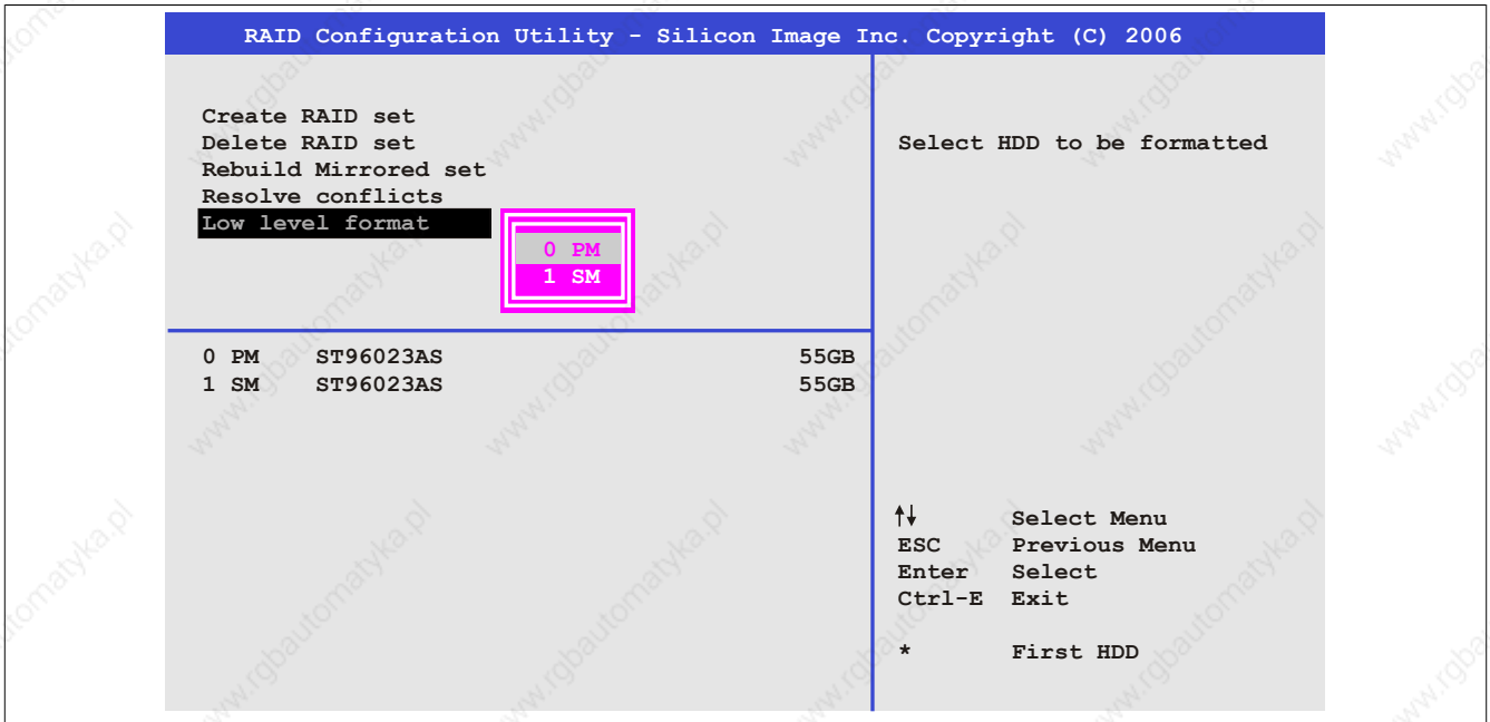
Figure 111: RAID Configuration Utility - Low level format
