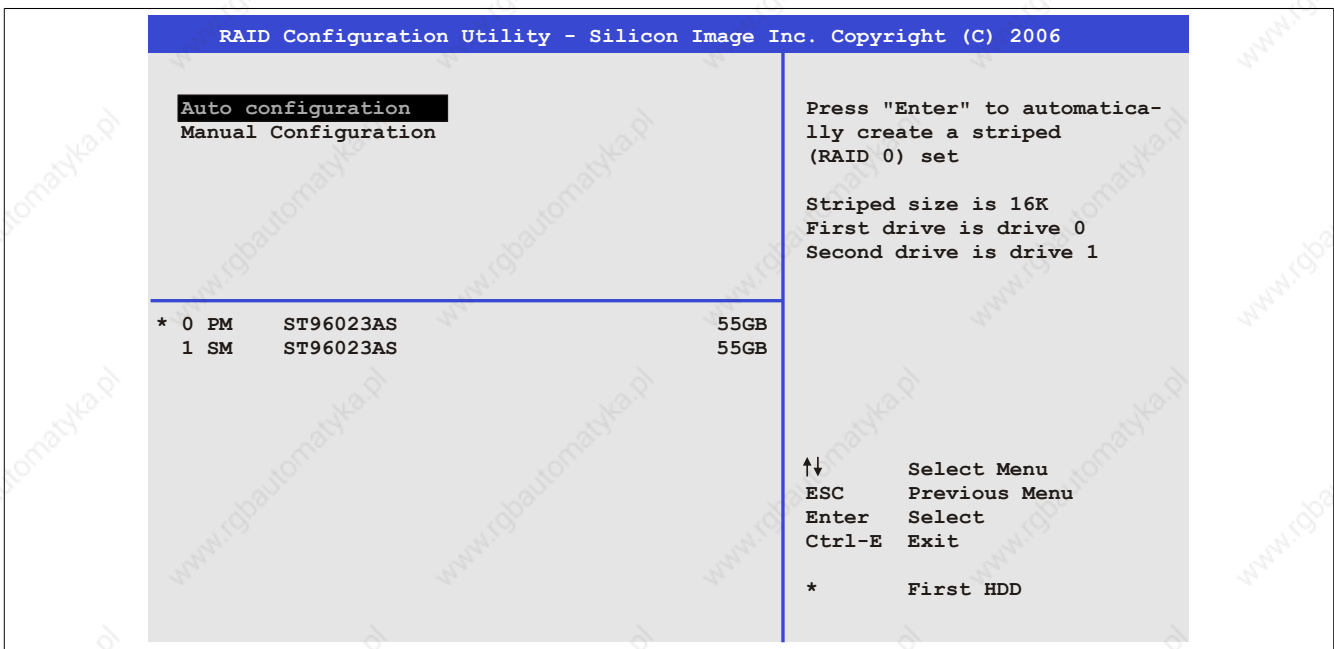
Figure 106: RAID Configuration Utility - Create RAID set - Striped
