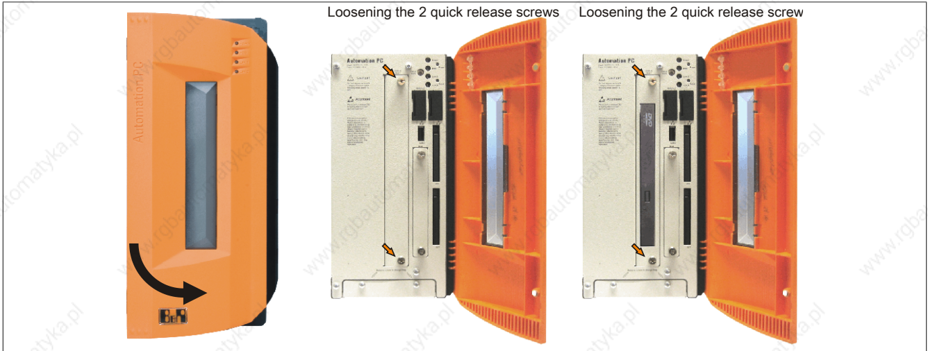
Figure 231: Loosening the quick release screws
