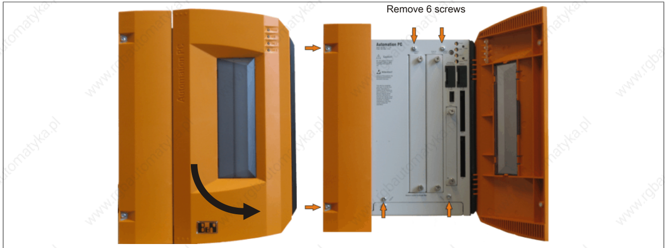
Figure 280: 5-slot APC810 - Installing the side cover
