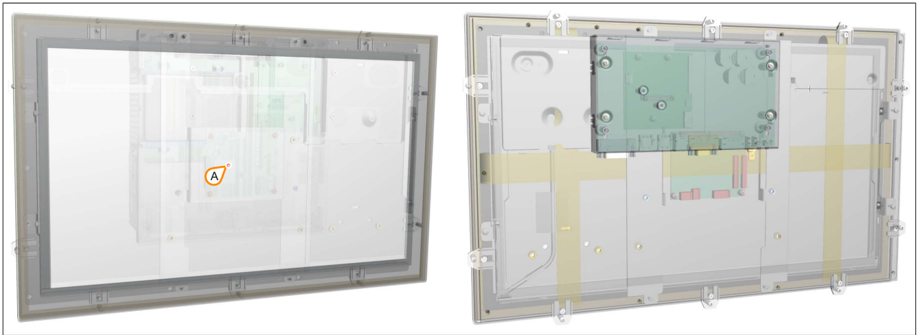
Figure 7: Automation Panel 9x3 - Temperature sensor position
