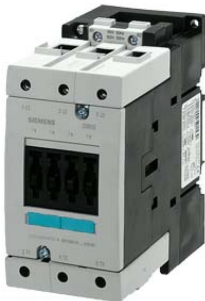
CONTACTOR, AC-3 30 KW/400 V, DC 220 V, 3-POLE, SIZE S3, SCREW CONNECTION
