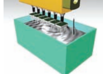
Inspecting the solder level in soldering tanks
