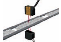
Checking for doubled-up lead frames
