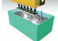
Inspecting the solder level in soldering tanks
