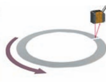
Checking welding point positions on ring gears
