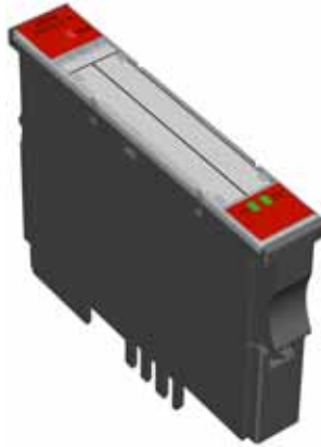
Figure 90: Digitale output module, 2 digital outputs, 24 V DC, 2 A, positive switching
