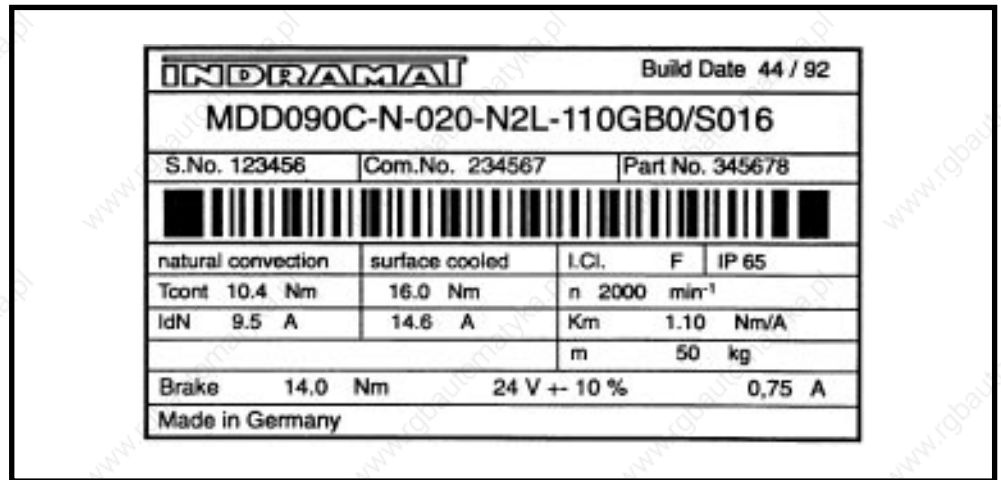
Fig 15.2: Example of a name plate of an MDD AC servo motor per DIN 42961
