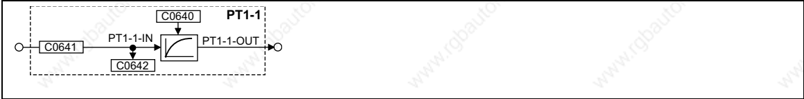
Fig. 3-144 Delay element (PT1-1)
