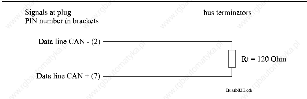
Fig. 48: CAN bus terminators
