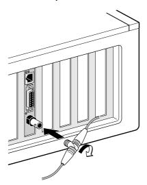
2 Connect the other end of the network cable to another PC or to a 50-ohm terminator.
