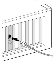
2 Connect the other end of the network cable to an active network port.
