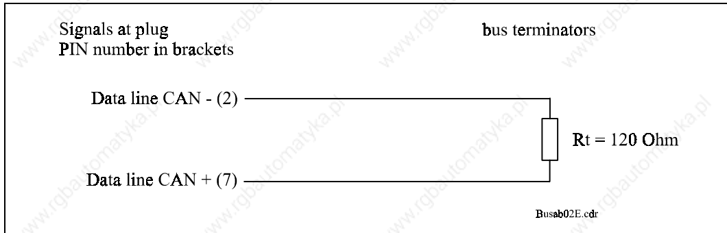
Fig. 48: CAN bus terminators
