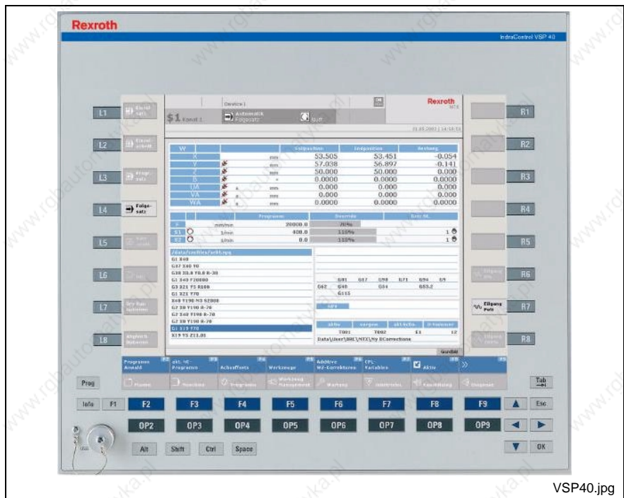
Fig. 5-2: VSP 40.1 with 15" color display
