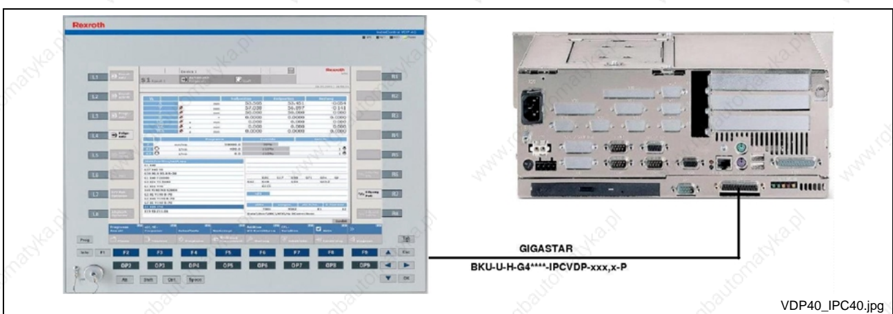
Fig. 8-2: High-end industrial PC IPC 40.2/VPB 40.1 with operator panel VDP 40.x
