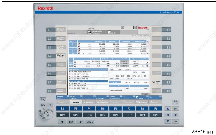
Fig. 5-1: VSP 16.1 with 12" color display
