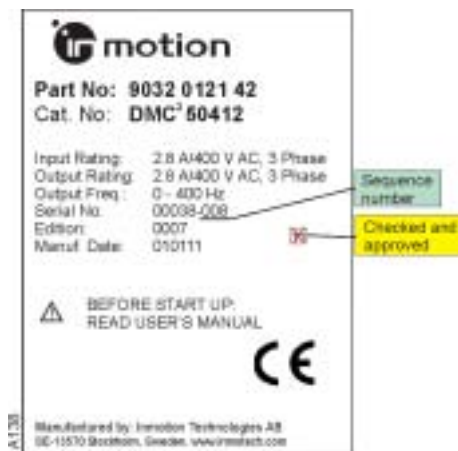
Figure 2. DMC 2 Product Identification Label.
