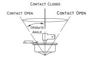
Tip-Over Switches operate when the switch is tilted from the vertical position. The angle through which the switch has ti move before operating is called the operating angle. These switches are omni-directional.
